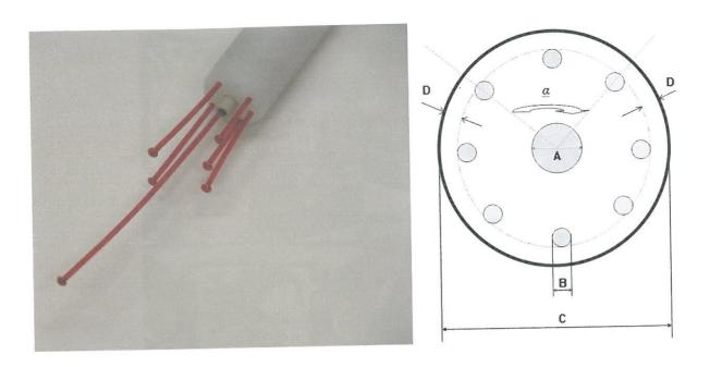
**Figure 7.** Close image of the device with applicators and schematic drawing. On the diagram diameter of the central canal (A = 5 mm), of the circumferential channels (B = 2 mm) and of the whole vaginal cylinder (C = 23 mm) is presented. The circumferential channels are drilled at a distance (D) of 2 mm-s from the surface and the angle  $\alpha = 90^{\circ}$ .
